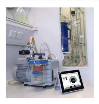
Convenient control down to 10 <sup>-3</sup> mbar Complete packages provide everything you need for controlling vacuum down to 10 <sup>-3</sup> mbar.
