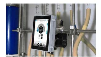
All-in-one, when and where you need it The VACUU ·SELECT Complete Controller includes the control module, and integrated vacuum sensor, control valve, and venting valve. Available with a table top stand, for lab scaffold mounting, or for panel mounting.
